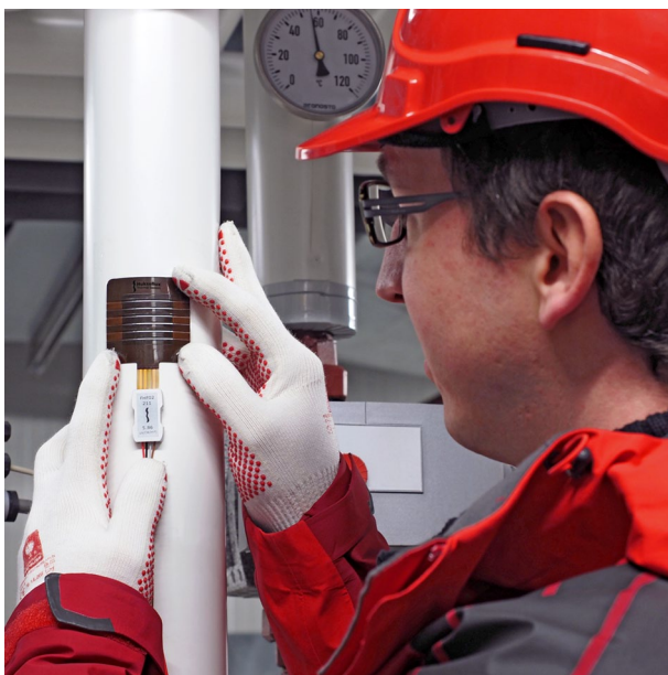
Figure 2 FHF02 being installed on a pipe
