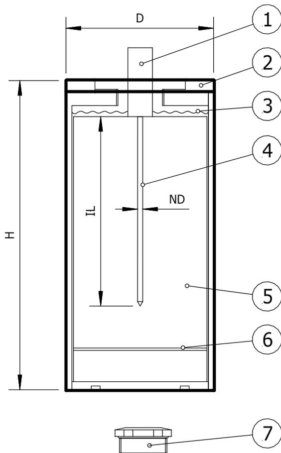
The heart of the CRC cylinders is a specially manufactured amorphous plastic reference material (5). Contrary to other plastics, this material does not have any directionally dependent thermal properties.
